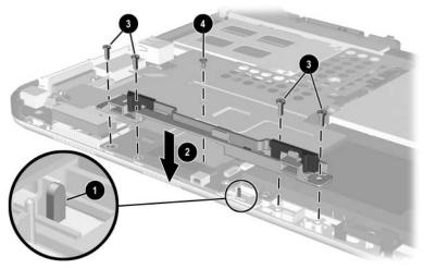
Installing the Keyboard Release Assembly
